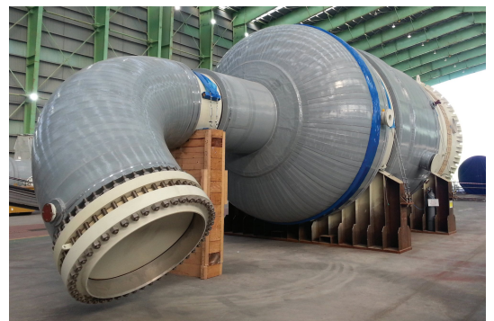
Vessel Insulation for FLNG Top Side
